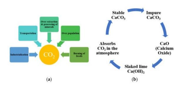
Lime is one of the most sustainable materials in existence today, it can be used over and over again without losing its integrity or quality. Lime mortars have proven themselves to be durable materials with great potential for longevity and lime absorbs CO2.
